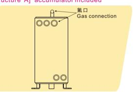
自带储液罐可有效降低氟系统压力,提高换热效率。 When there is accumulator included, the gas pressure of the heat pump can be reduced obviously, thus enhance the heat exchanger efficiency.
